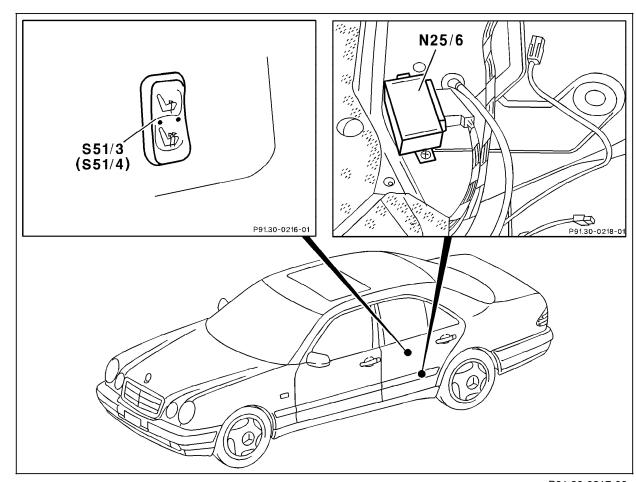
N25/6 Rear HS control moduleS51/3 Left rear seat heater switchS51/4 Right rear seat heater switch
