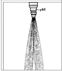
Figure 1 Y62 Injector Good spray pattern
