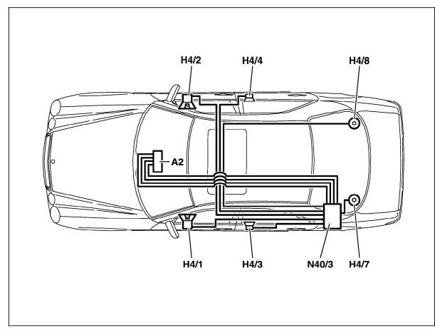
Figure 1 Model 210.0 with Sound System
